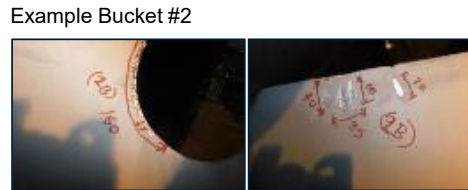
Example Bucket #2 Inspection 04.09.18 6642 operating hours
